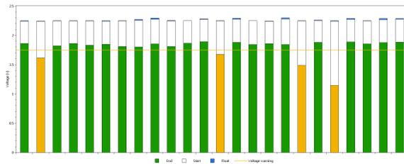
Figure 3: Test 3, Individual Cell Voltages (4-Hr Test)
