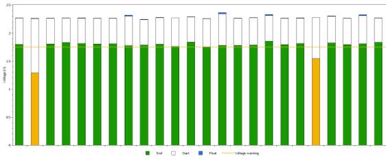
Figure 1: Test 1, Individual Cell Voltages (1-Hr Test)
