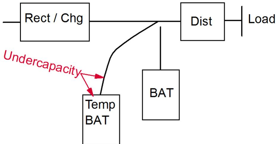
**Figure 1. Under-capacity temporary battery or cabling often cause failures.**
