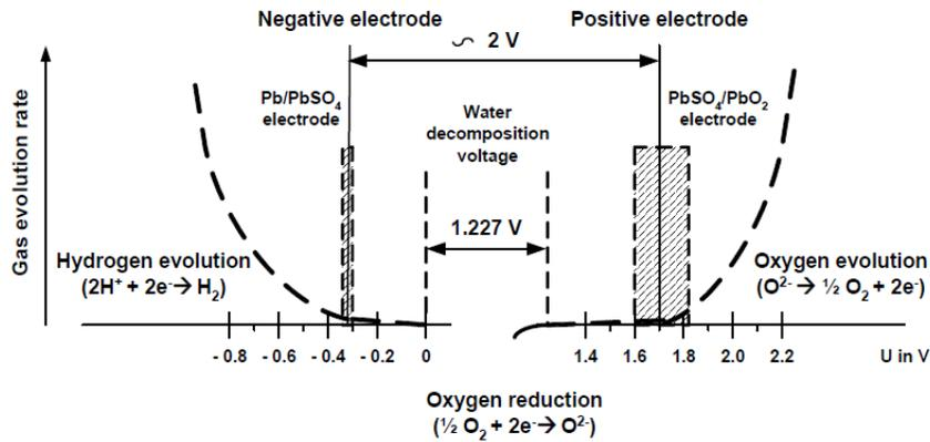
**Figure 4. Water decomposition increases markedly as the voltage difference between the positive and negative electrodes (plates) increases.**
