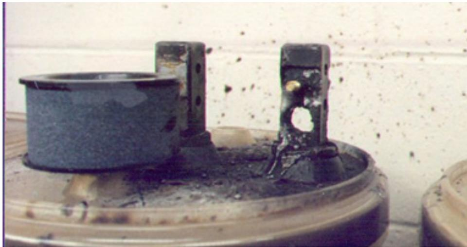
Figure 2. This photo shows a post meltdown due to a resistive intercell connection and a battery discharge.
