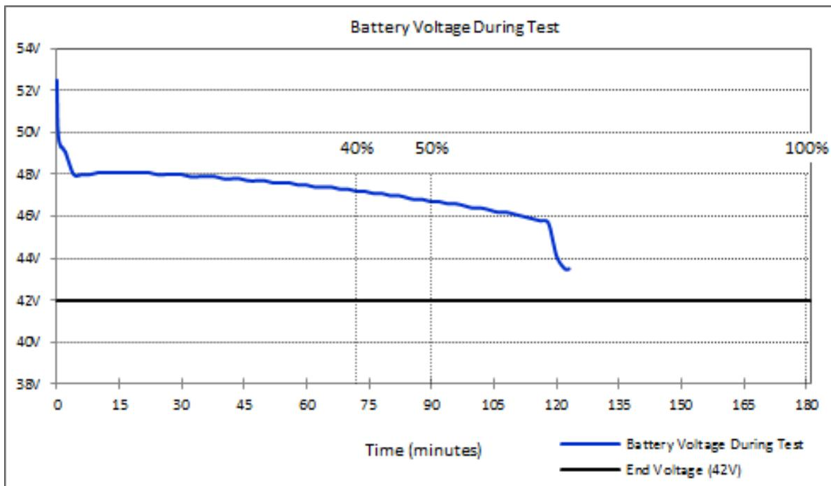
Figure 8. Impact of one defective cell that failed 120 minutes into a 180 minute test<sup>iii</sup>.
