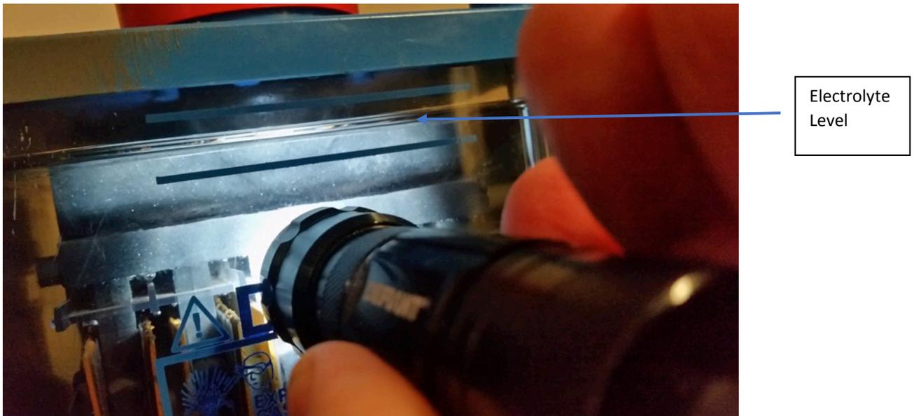
Figure 1. Light Below the Liquid Level
