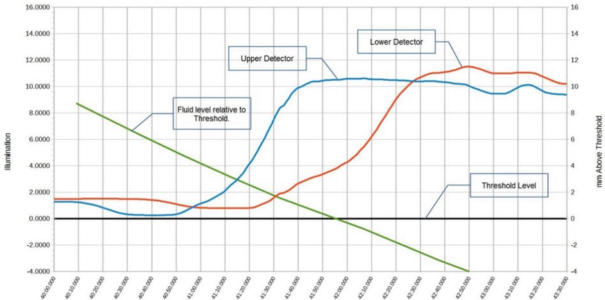
**Figure 4. Graph of IR Receiver Output Samples for the Two Detectors as the Electrolyte Level Falls**
