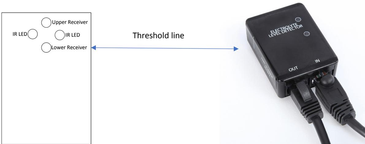
**Figure 3. Optical Placement Diagram for the Infrared Level Detector**
