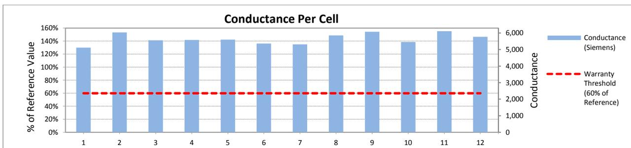
**Figure 3. Ohmic Readings**
