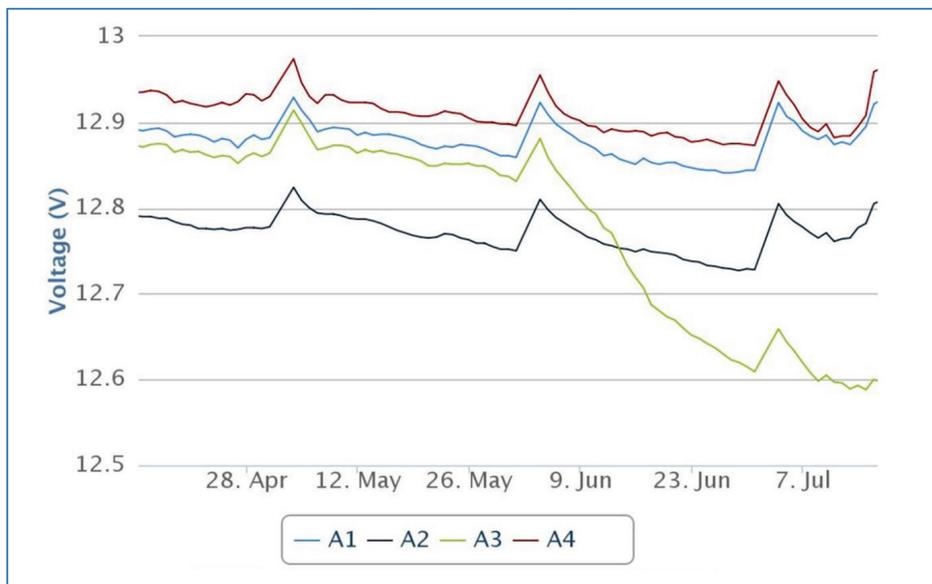
**Figure 4. Example of OCVs of a string of batteries. Battery A3 is defective due to a manufacturing defect.**
