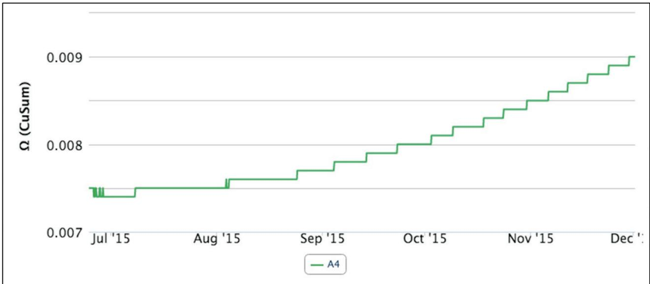
**Figure 3. Change in DC resistance with time for a VRLA battery in a 48V string. The plot shows resistance in mΩ vs date.**
