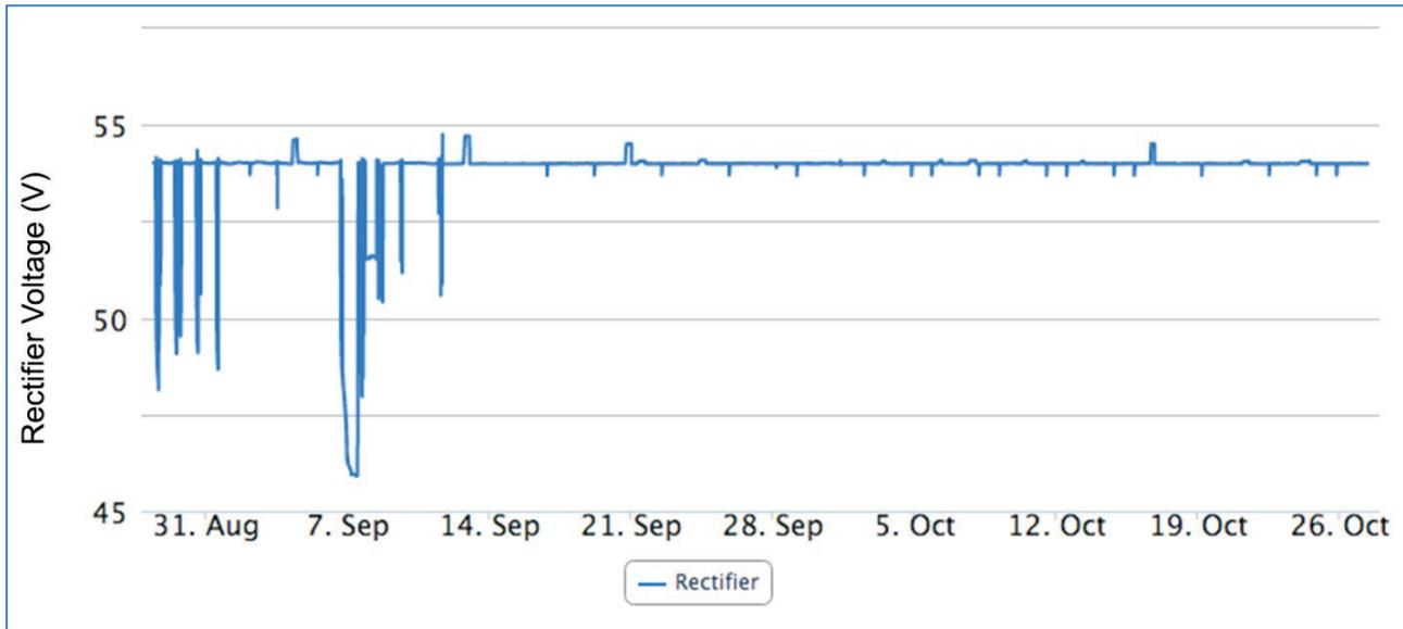
Figure 2. Example of power outages for Company A. The plot shows the rectifier output voltages vs date.
