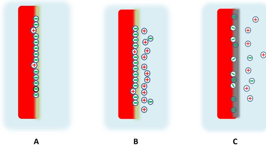
Figure 6: Double layer capacitance in lead-acid cells
