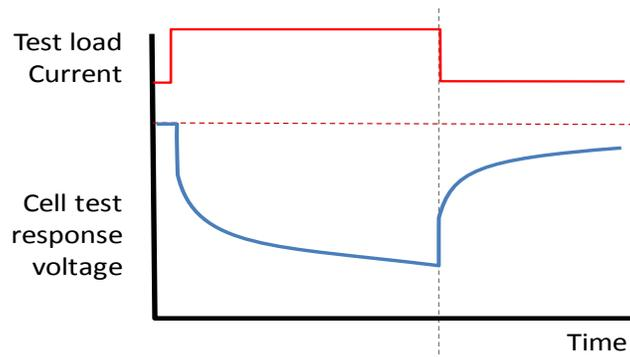
**Figure 9: Testing an on-line lead acid cell**
