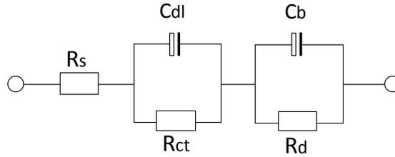
**Figure 8: Expanded equivalent circuit for a lead-acid cell**
