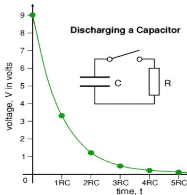
**Figure 4: Characteristic voltage curve of a discharging capacitor** (Graph: Schoolphysics.co.uk)
