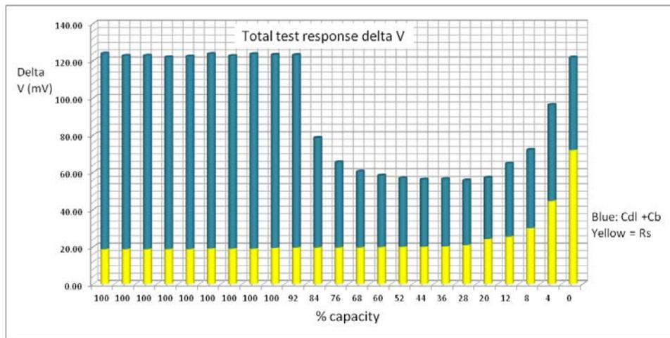
**Figure 16B: Capacitance-resistance test voltage deltas from VRLA monobloc #2**
