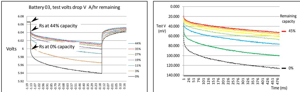
**Figure 15: Increase in test response voltage due to increase in Ohmic resistance**
