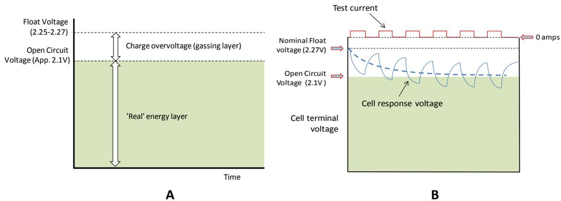
**Figure 10 A: Float charge overvoltage** **Figure 10B: Ineffective low-current testing**
