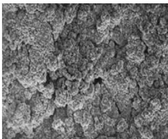
**Figure 17A: New plate, with no sulphation.**
