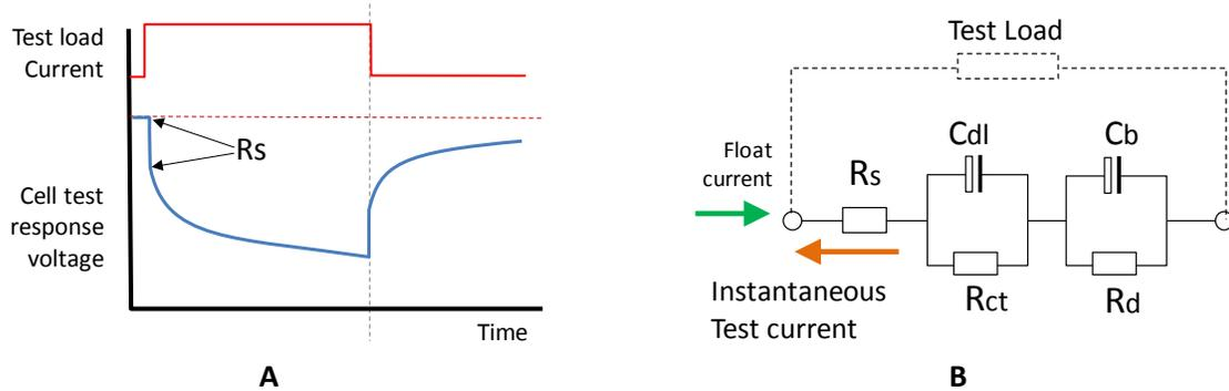
**Figure 11: The vertical section of the voltage response proportional to internal resistance**
