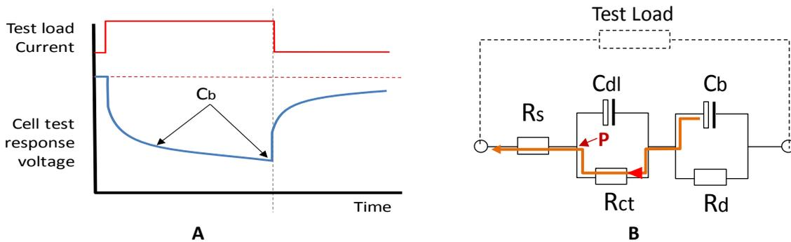
Figure 13: The bulk capacitance linear response section
