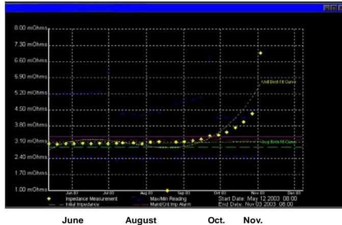
Figure 2: In-service battery impedance at end of life Graph courtesy of Btech Inc.
