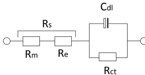
**Figure 1: The Randles equivalent circuit for a lead-acid cell**
