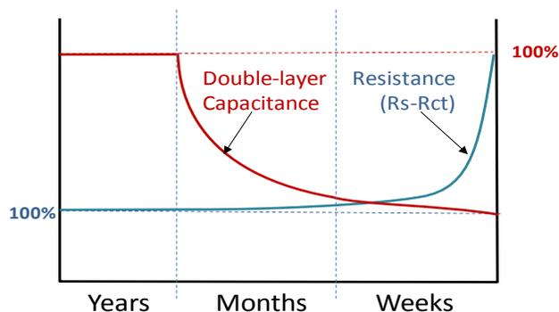
**Figure 7: Idealised lifetime resistance and capacitance characteristics for an L-A cell**
