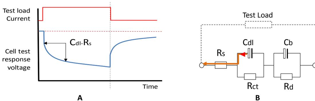
**Figure 12: The  $C_{dl}$  discharge curve**
