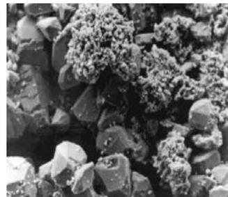
**Figure 17B: Plate from undercharged cell after less than one year, with pronounced sulphation.**
