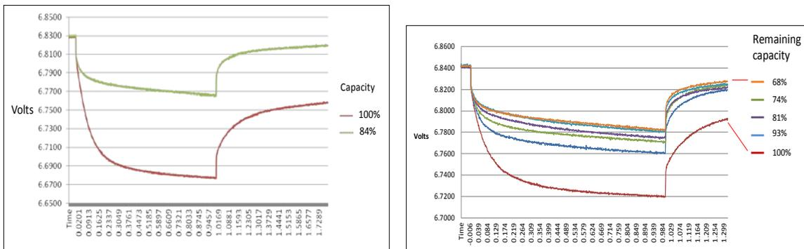
Figure 14: Reduction of depth of Cdl-Rs curve of VRLA monoblocs at different capacities
