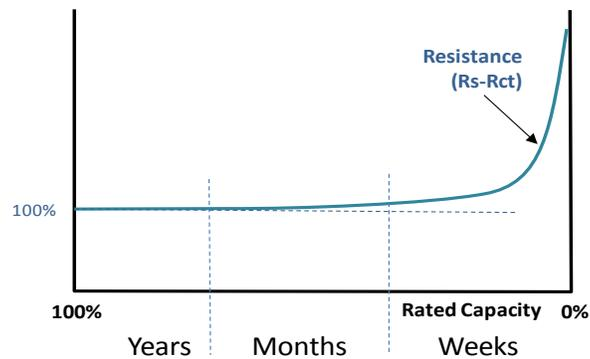
Figure 3: resistance/impedance curve of a lead-acid cell over service life
