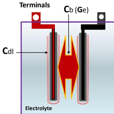
Figure 5: The two most significant capacitances occurring in a lead-acid cell, Cdl and Cb (Ge)
