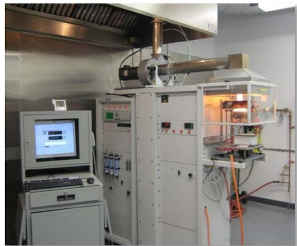
**Figure 3. Schematic layout of a cone calorimeter (left) and Exponent's cone calorimeter (right).**
