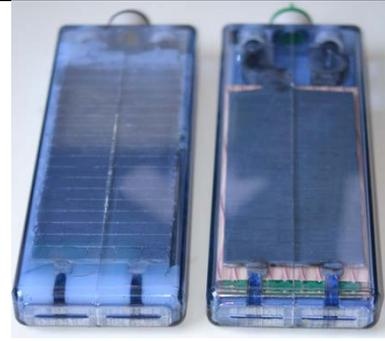
**Figure 3. Special built test cells. Left: sealed design with gelled electrolyte (OPzV). Right: vented design (OPzS)**
