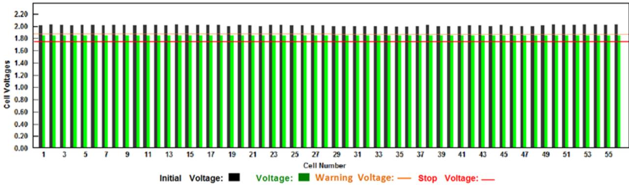
**Figure 4: Initial and final voltage of each cell with warning and stop limits**
