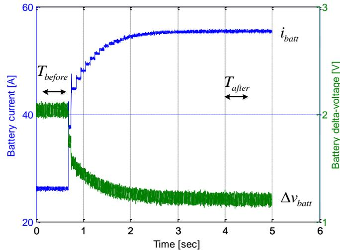
**Figure 2. Typical result from a recorded step test for evaluation of the internal resistance**
