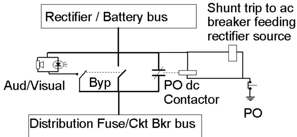
**Figure 8. A zoned power disconnect arrangement with a bypass feature for system tests**
