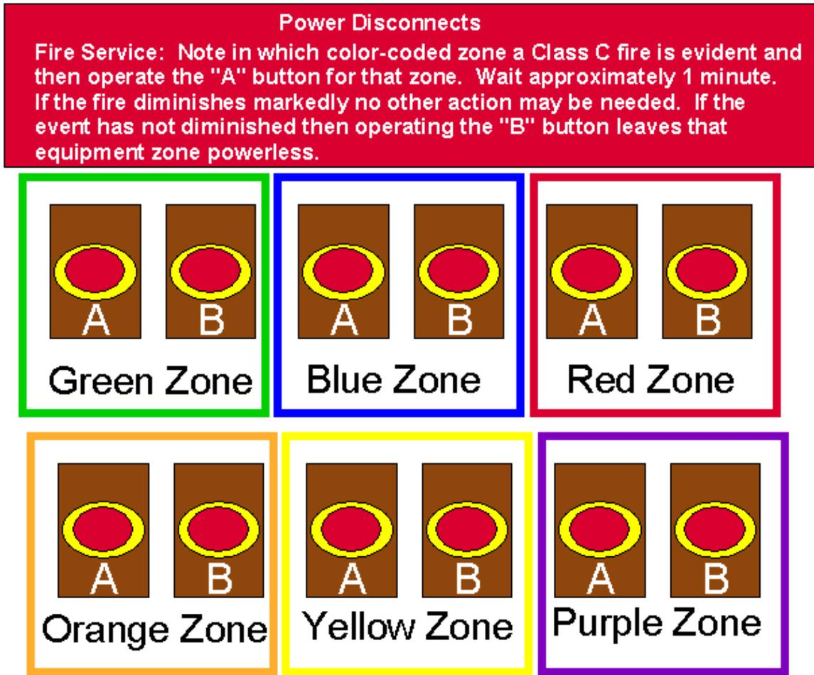
**Figure 7. A zoned power disconnect arrangement for facilities with distributed dc (6 zones are shown in this example).**
