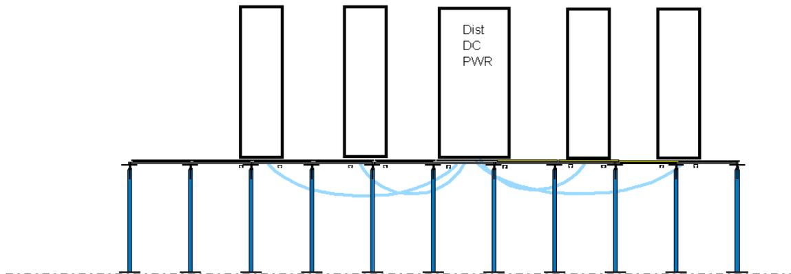
**Figure 9. End view sketch of rows showing -48 volt feeding cabinets via flexible conduits.**
