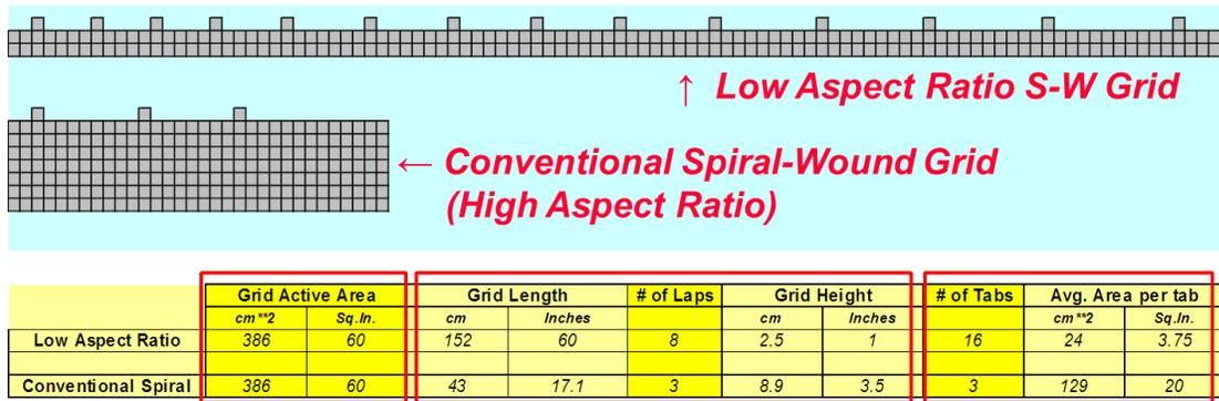
**Figure 2. Spiral-Wound Grid Comparison: LAR-VRLA Grid vs. Conventional VRLA Grid**
