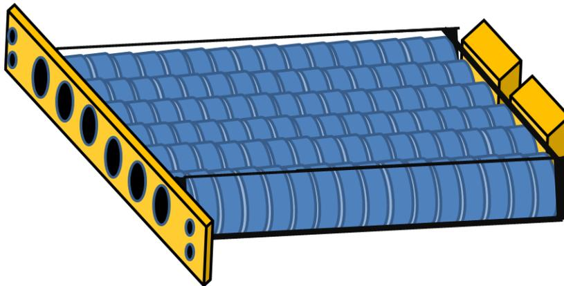
**Figure 6. Rack-mounted air-cooled low aspect ratio VRLA battery pack**
