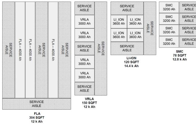
**Figure 5. Battery Layout Space Comparison**
