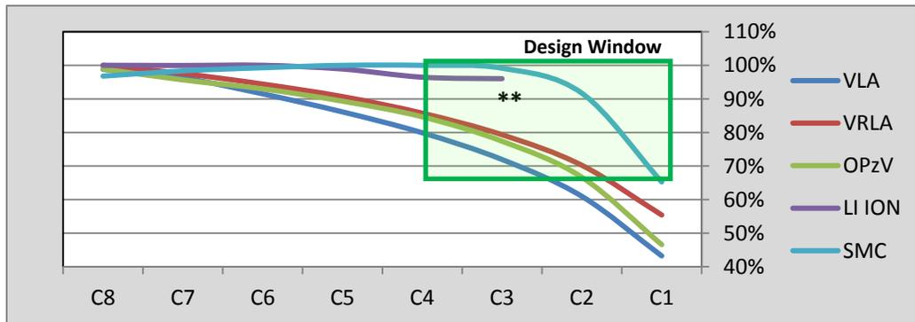
**Figure 6. Discharge Performance(C Rate) vs Percentage of Capacity Rating**
