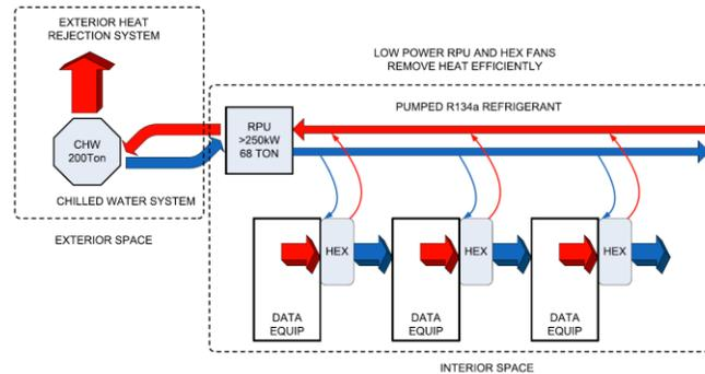
**Figure 9. Refrigerant Based Direct Cooling System Design**
