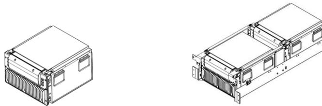
**Figure 7. SMC 48V / 200Ahr and 400Ahr bolt-in Shelf Assembly**
