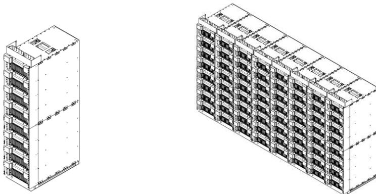
**Figure 8. SMC48/3200Ah Group and 25.6 k Ah System**
