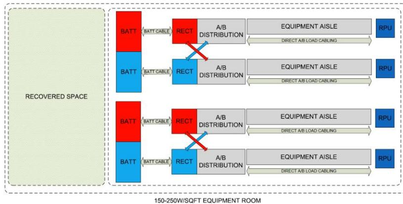
**Figure 3. Direct Distribution Facility Design**
