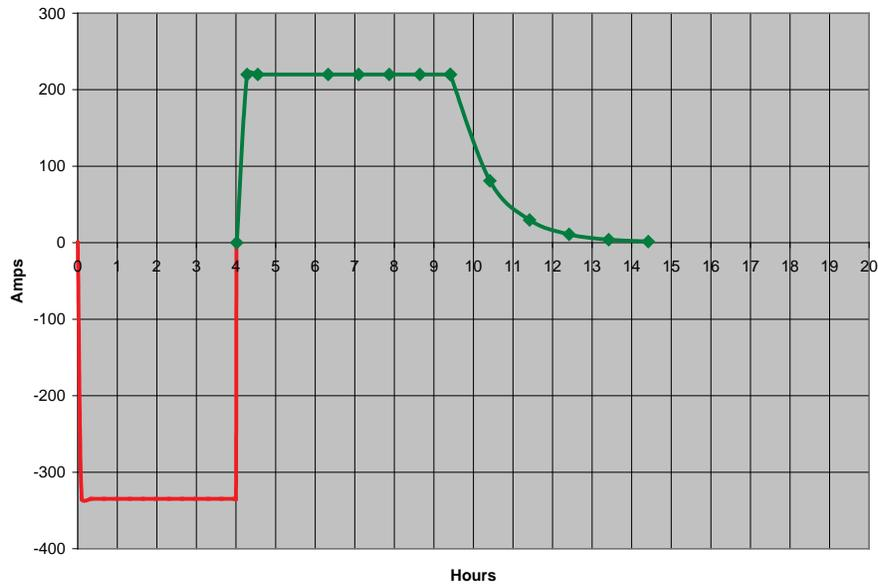
**Figure 5 – 4-hr Duty Cycle Discharge, Charge at Equalize**
