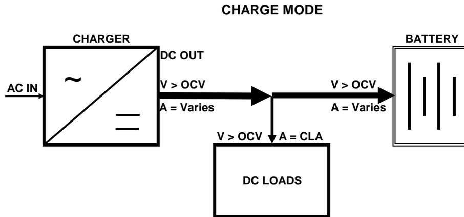
**Figure 4 – Battery System in Charge Mode**
