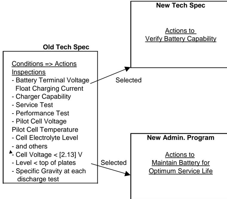
Figure 1 – Separating Capability and Maintenance
