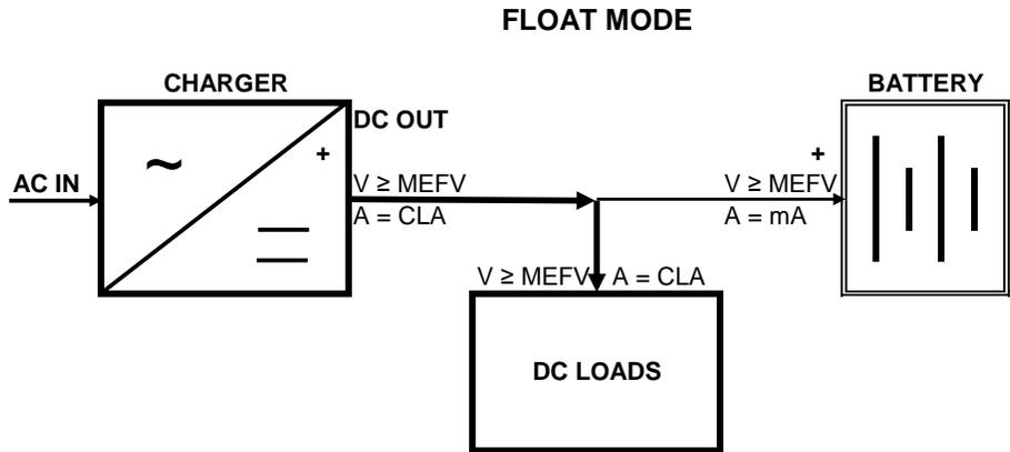
**Figure 2 – Battery System in Float Mode**
