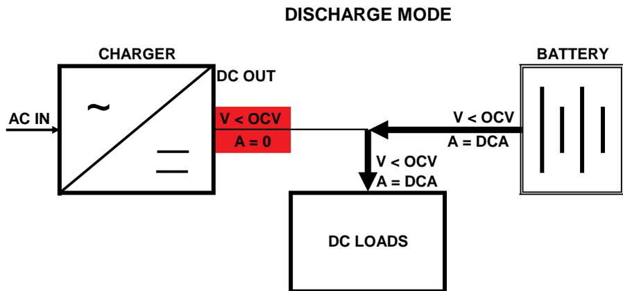
**Figure 3 – Battery System in Discharge Mode**
