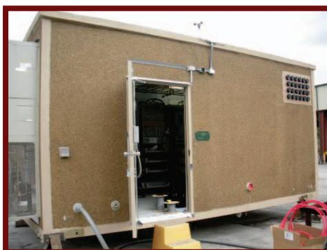
Figure 6 – Smoke and Hydrogen Detection Test Structure
