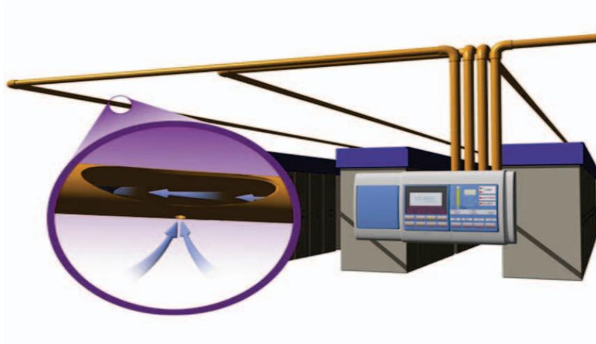
**Figure 4 – Air-Sampling Smoke Detector**
