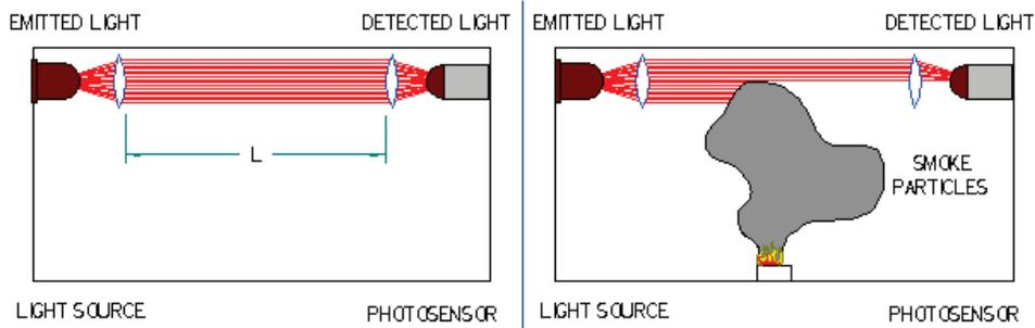
**Figure 3 – Projected Beam Smoke Detector**
