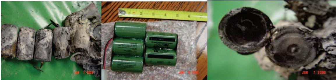
**Photos taken by PHMSA inspectors as part of their investigation into a reported battery fire in a small parcel air carrier facility.**
