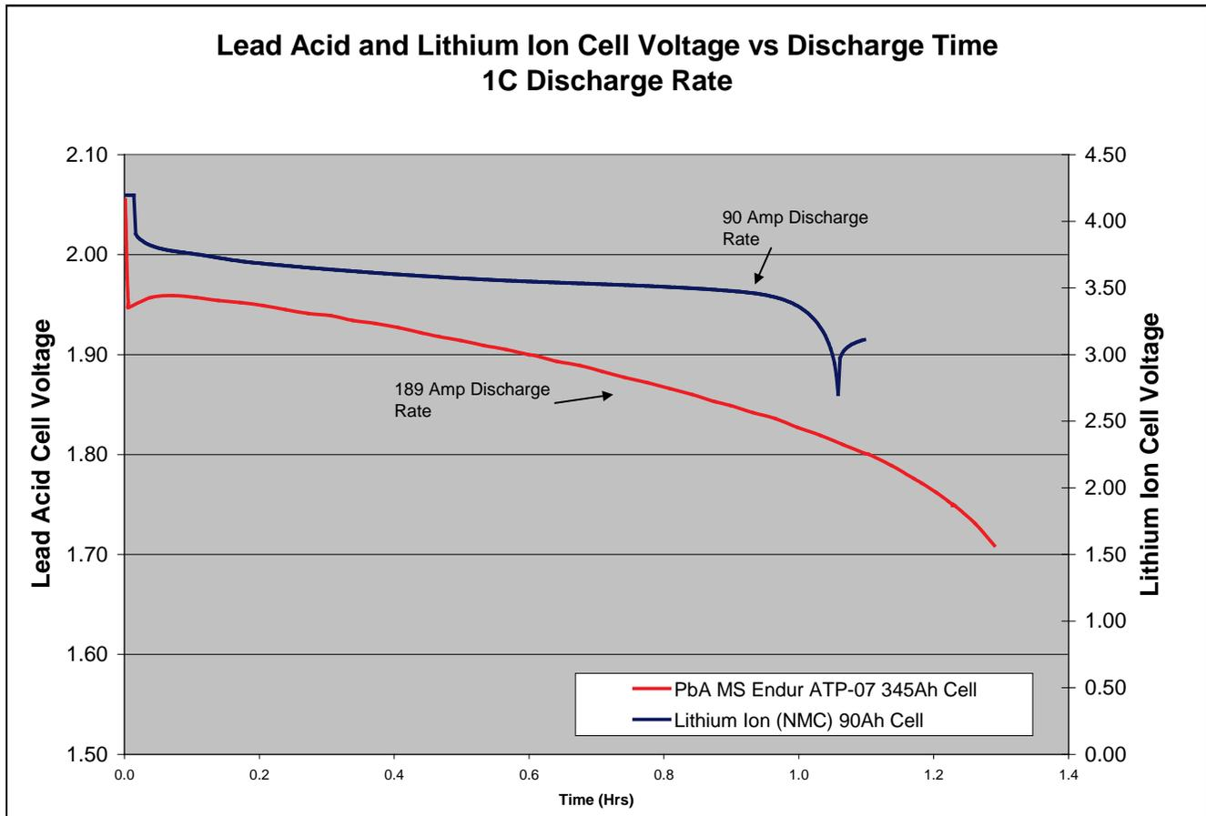
Figure 5. Discharge Curve Comparison: Lead Acid versus Lithium Ion
