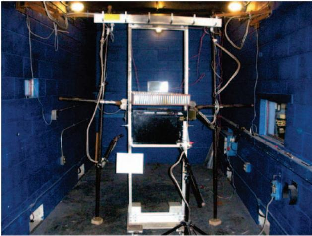
**Figure 8. NEBS Fire Resistance Test**
