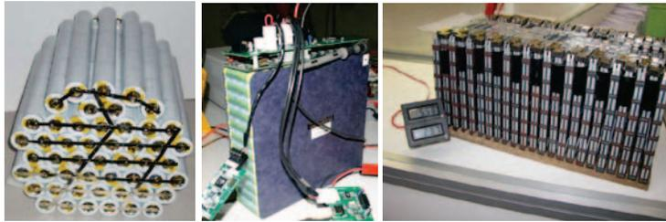
**Figure 6. Large Cell Count Battery Packs With Numerous Connections**
