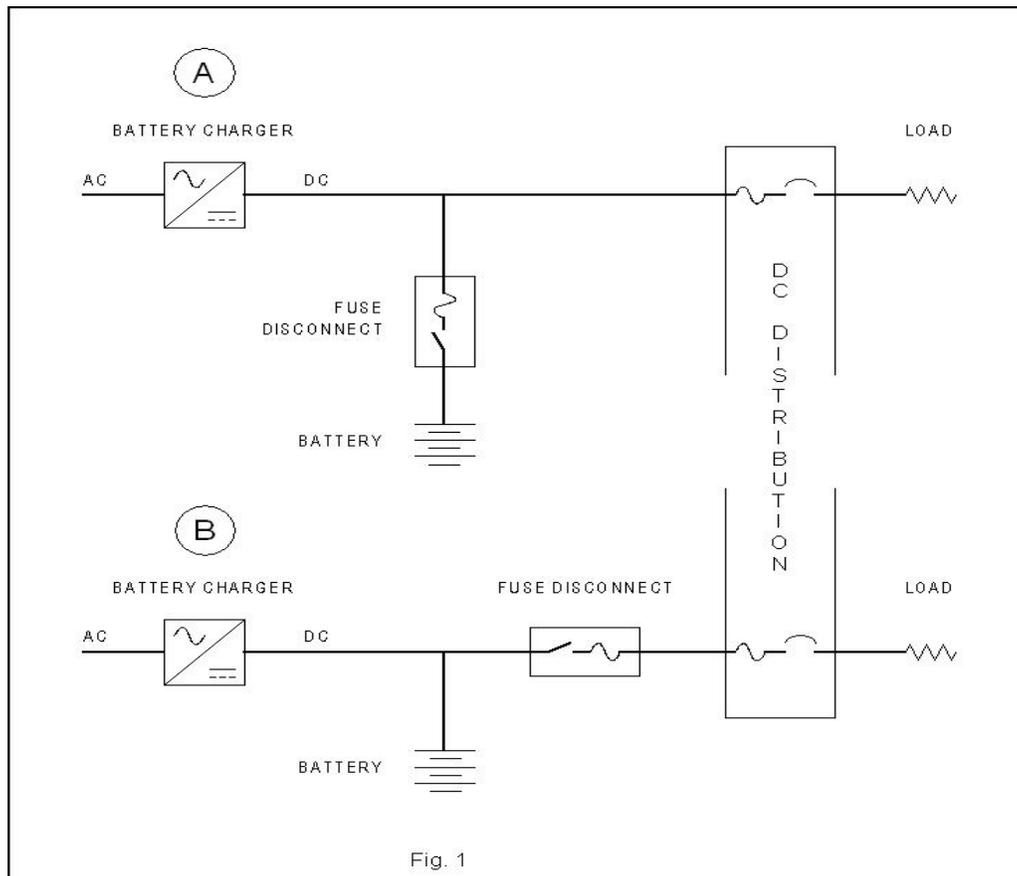
One line diagrams of a simple dc bus
