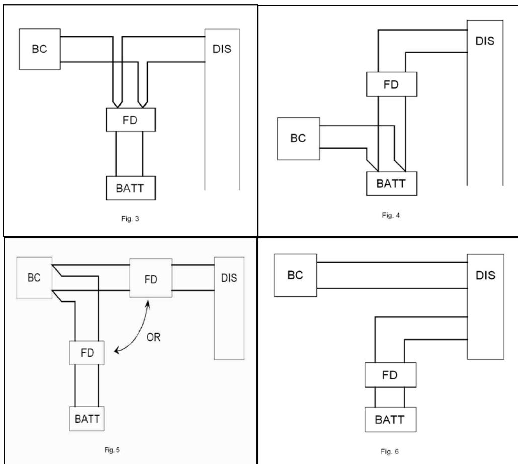
**FD=Fused Disconnect BC=Battery Charger DIS=Distribution panel**
