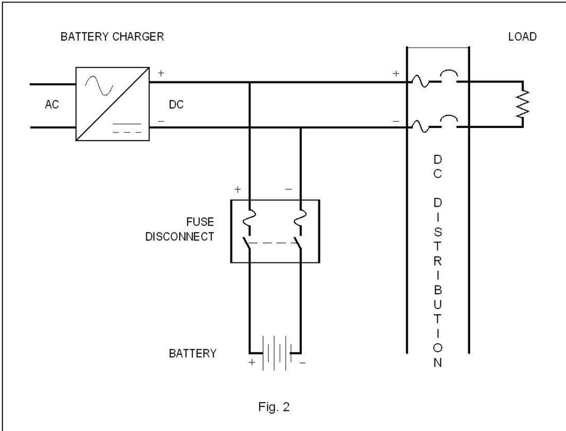
The two line of Figure 2 shows a clearer view of the electrical connections, but not the wire connections.
