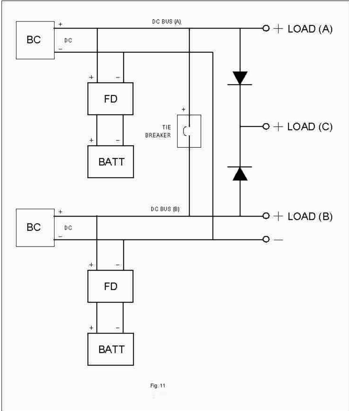
**Dual battery chargers and batteries with three loads**
