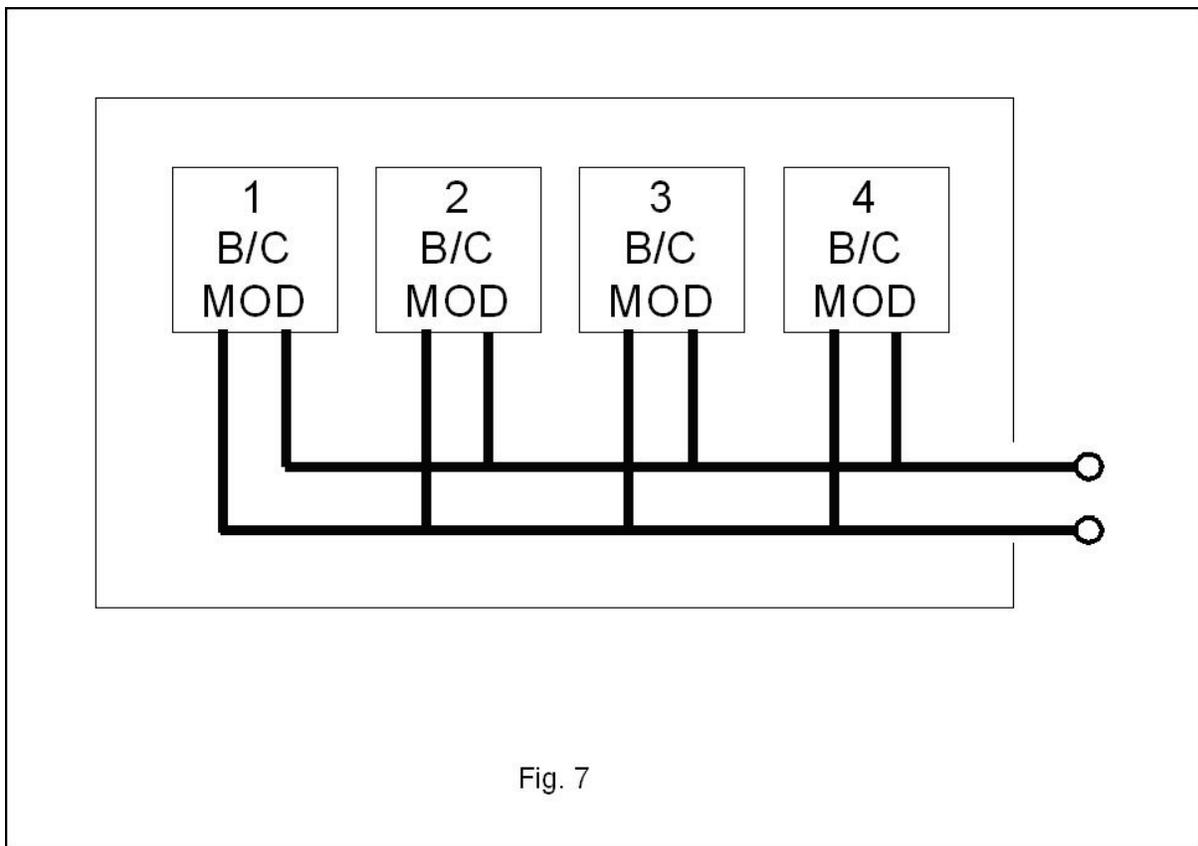
**Paralleled battery modules wired in a backplane for redundancy**
