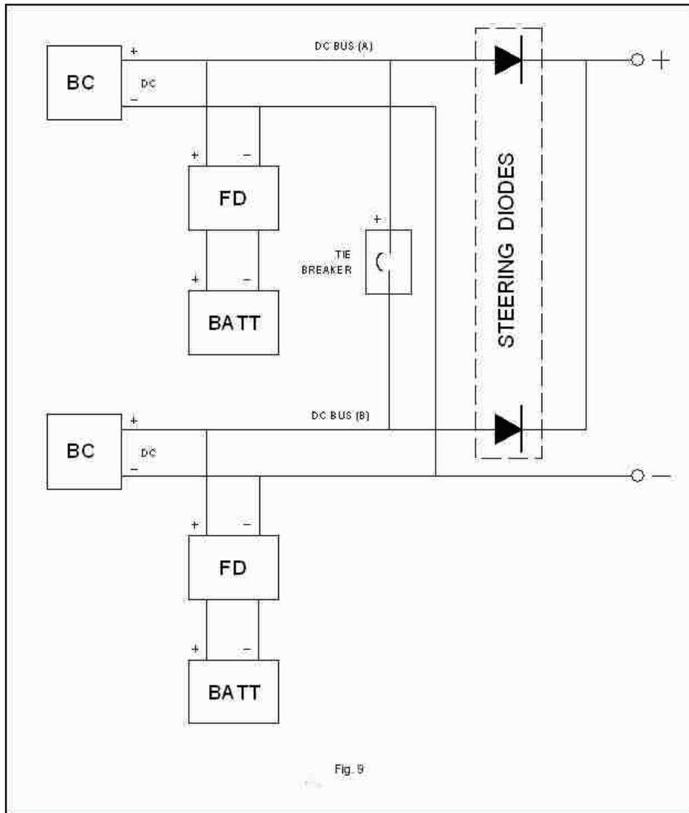
**Dual batteries and battery chargers with steering diodes**
