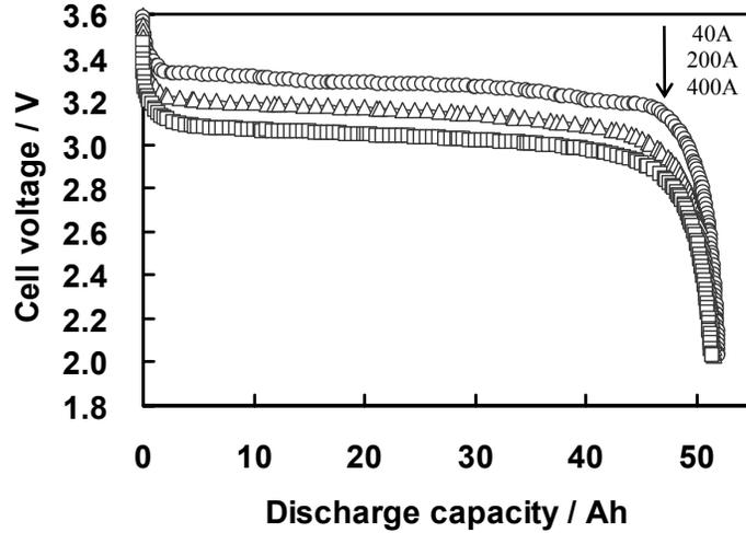
**Fig. 9 Discharge Voltage Profiles of Improved Fe Large Cell at Various Discharge Rates**
