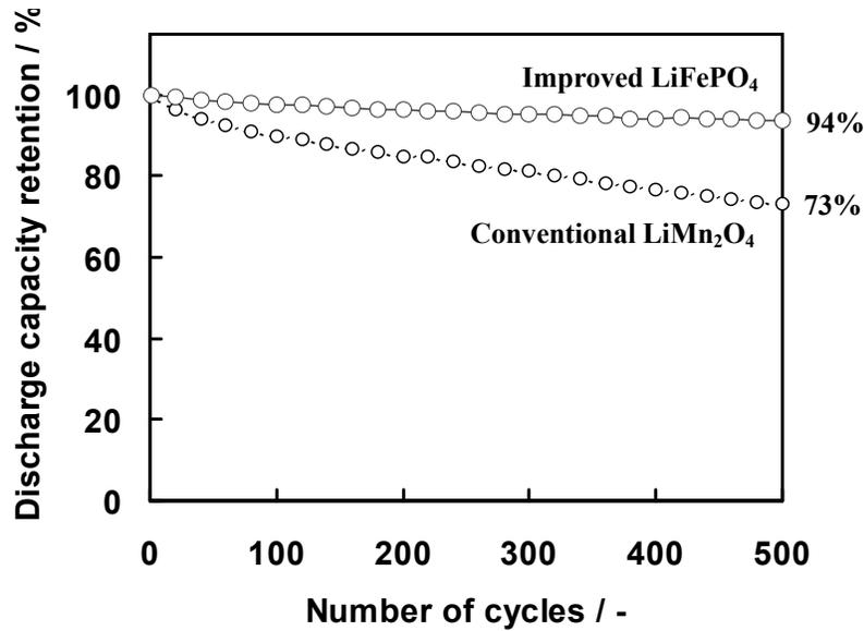
**Fig. 7 Cycle Life Test Results of the Improved Fe Small Cell and the Conventional Mn Small Cell at 45 °C**
