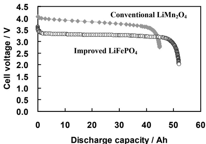
**Fig. 8 Discharge Voltage Profiles of Improved Fe Large Cell and Conventional Mn Large Cell**
