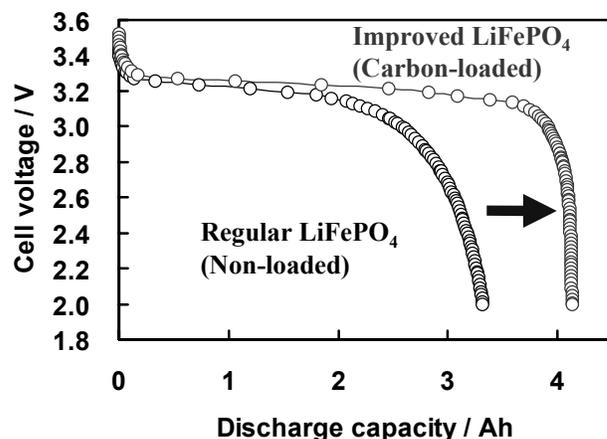
**Fig. 4 Discharge Voltage Profiles of Regular Fe Small Cell and Improved Fe Small Cell**
