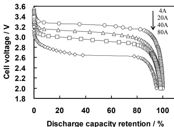
**Fig. 5 Discharge Voltage Profiles of Improved Fe Small Cell at Various Discharge Rates**
