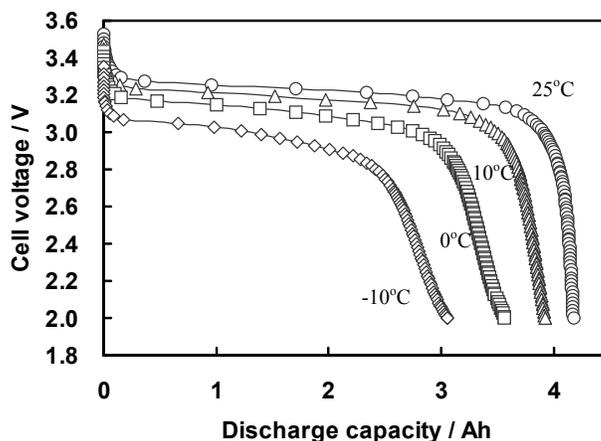
**Fig. 6 Discharge Voltage Profiles of Improved Fe Small Cell at Various Temperatures**
