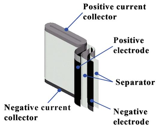
Fig. 2 Structure of the Small Cell
