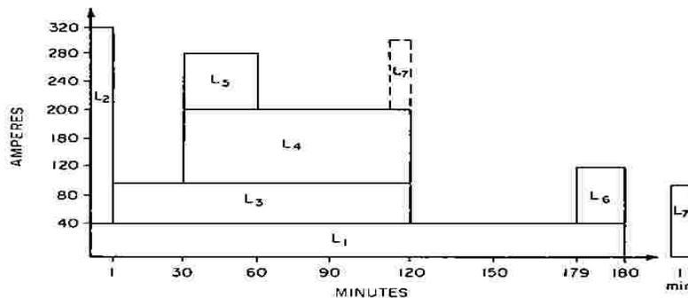
Figure 1 – Example of a complex duty cycle
