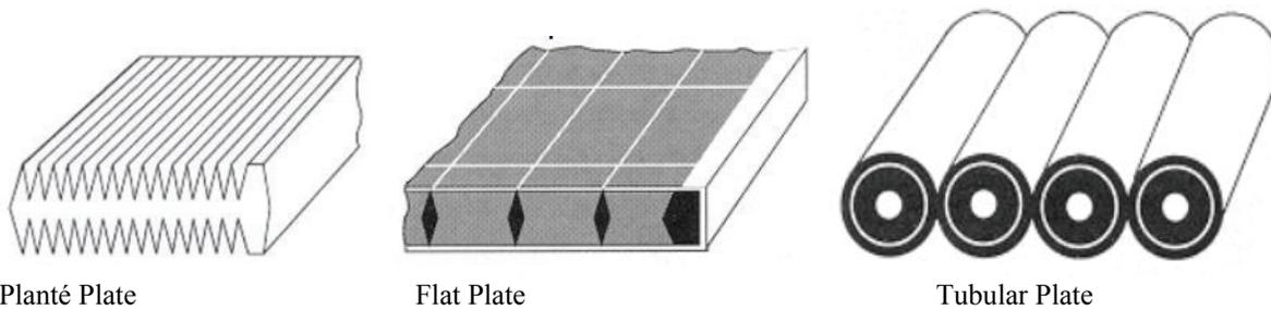
Figure 2 – Various plate designs for flooded lead acid batteries
