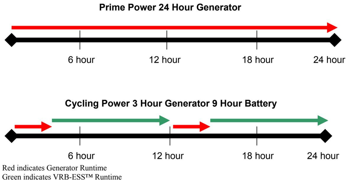
There is a concern that too much on and off cycling of the generators will lead to reliability problems. In order to reduce this to some agreed number of stop-starts, the VRB-ESS™ can be sized to have longer run hours by adjusting the electrolyte volumes. Additional storage costs less than a third of the system first cost so longer run hours are relatively inexpensive
