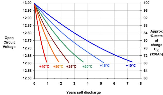
**Figure 2 – Self Discharge Characteristics of TPPL**
