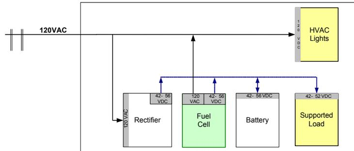
**Figure 1 – Typical Fuel Cell System Configuration**
