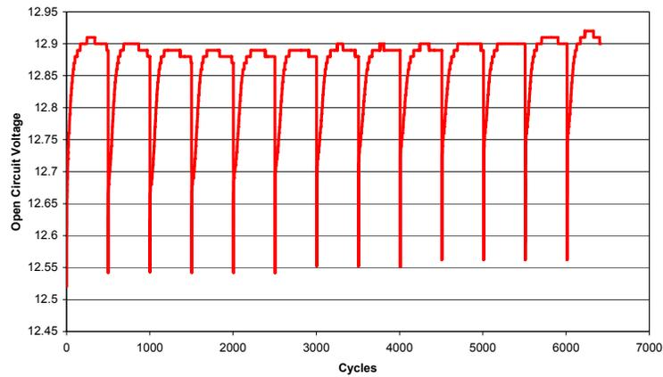
Figure 4 – Micro-cycle Testing of TPPL
