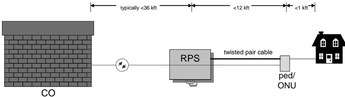
**Figure 3. FTTC powered from an RPS**
