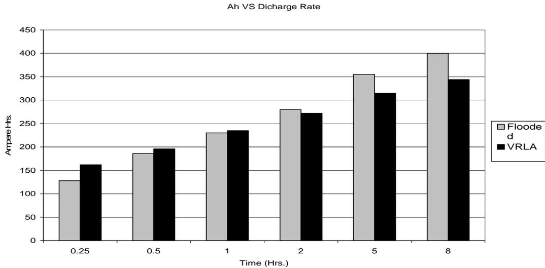
**Figure 1. AH VS Discharge Rate for Flooded and VRLA (400 Ah @ C/8).**
