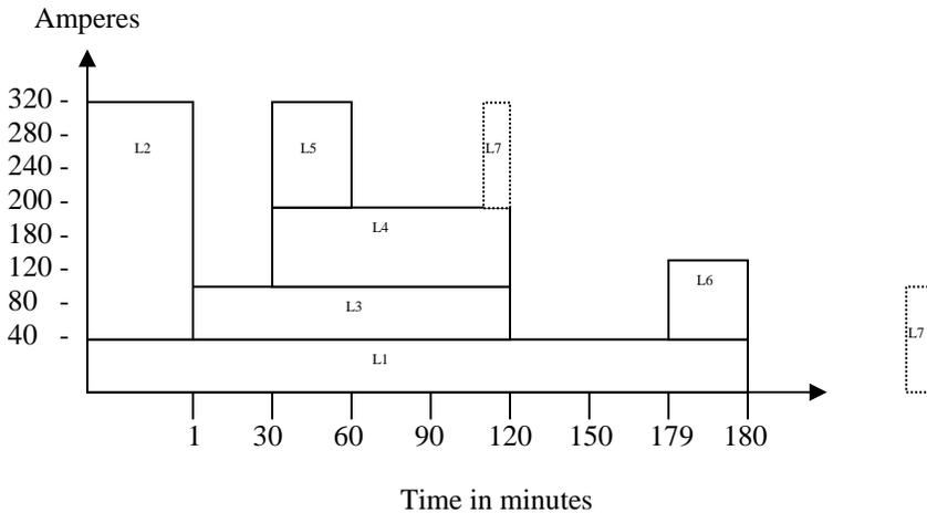
**Fig 2 - And then redrawn for sizing to look like this. This diagram provides for an easy way to accommodate the sizing process by listing the discharges as a serial list capable of being used by the sizing person.**
