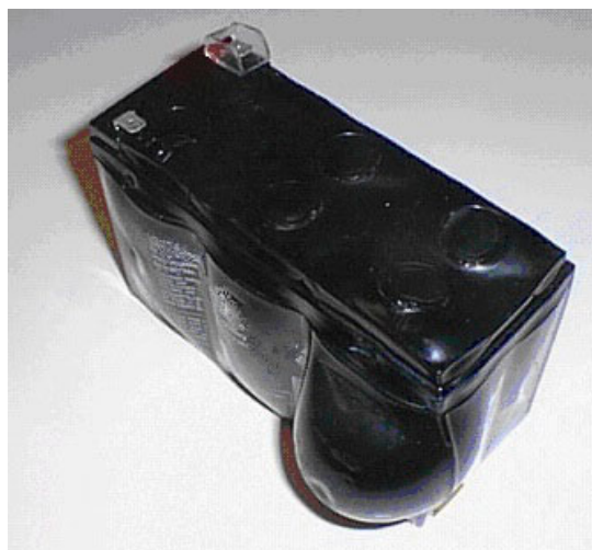
Figure 1. "Bloated" battery showing thermal runaway conditions
