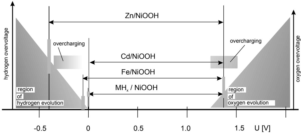
On extended overcharging, water from the electrolyte is decomposed, and there is hydrogen and oxygen evolution in faraday equivalent quantities. The water decomposition reactions seen at each individual electrode is shown in Figure 3.
