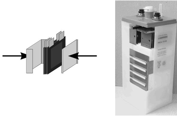
The design is based on the principle of a standard vented NiCd cell, with standard positive and negative electrodes. The plates are placed close together, and the electrode package is compressed between special plates to force oxygen between the electrodes. In addition, the design makes use of special non-woven separators that have been optimized to limit transfer of oxygen between the plates.
