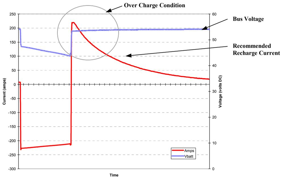
The test was then rerun utilizing the functions of the advanced controller. The controller was configured to perform a discharge test and to remove 20 percent of the battery capacity. The controller is capable of terminating the test when the desired capacity has been removed, or if other conditions exist including:
