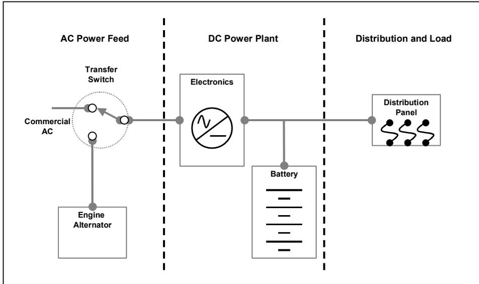
Reviewing published data on failures allows us to highlight the areas of the systems that are more susceptible. Table 1 summarizes the data published in *Network Reliability: A Report to the Nation*, which investigated the causes of network failures. As can be seen from the data, the failures are split evenly with one-third occurring in the AC Power Feed section, one-third occurring in the DC Plant section and one-third occurring in the Distribution and Load section.
