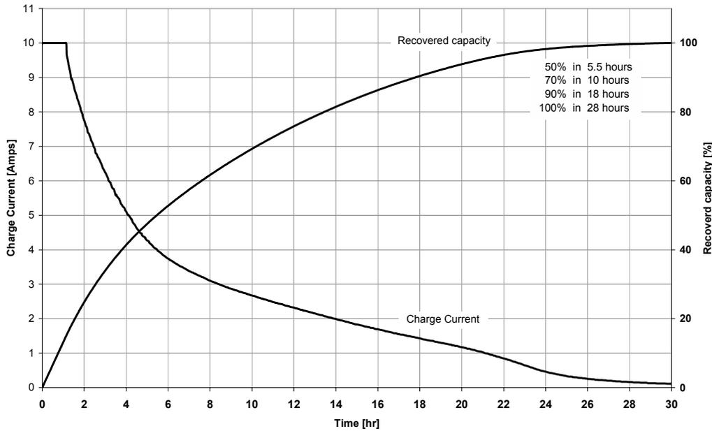
**Fig. 3 - Charge characteristic of a 48 V 80 Ah SMC battery**
