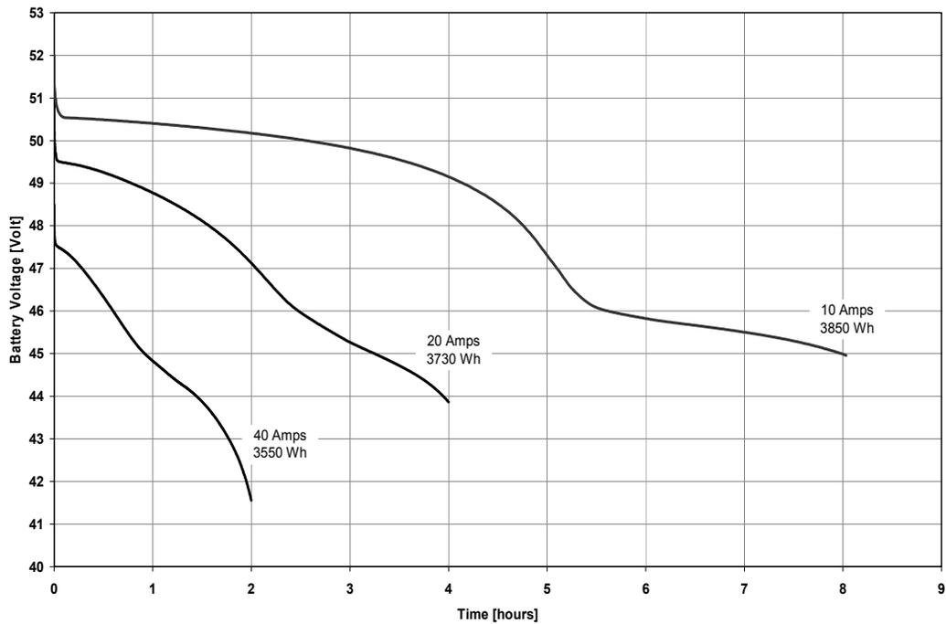
**Fig. 1 - Discharge curves of a 40 Volt 80 Ah Sodium-Metal Chloride battery at 275°C internal temperature**
