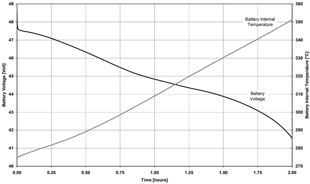
**Fig. 2 - Increase of the battery internal temperature during a discharge at 40 Amps (approx. two hour rate)**
