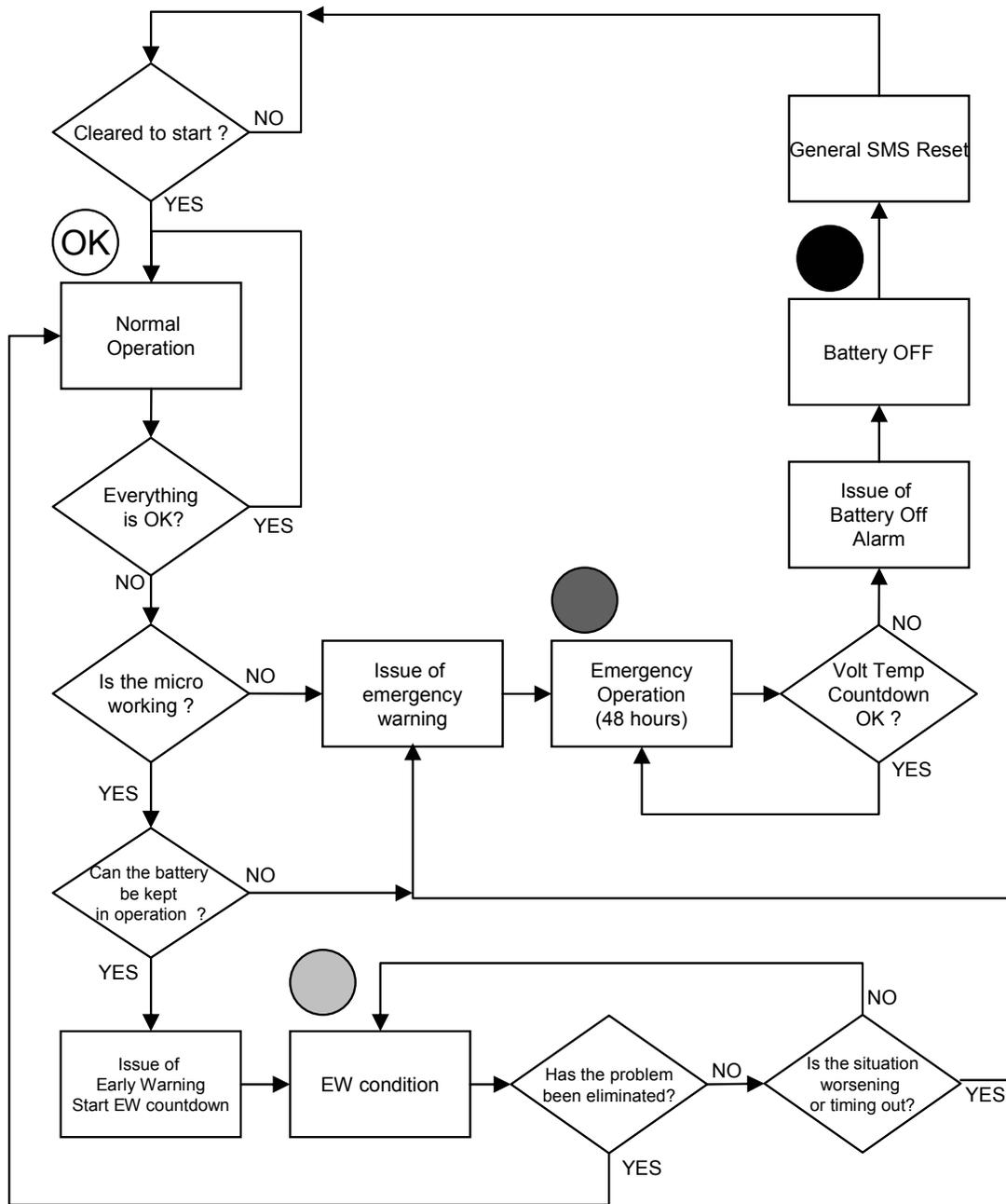
**Fig. 5 Flowchart of main loop of the battery management system with sequence of operations in case of failures.**
