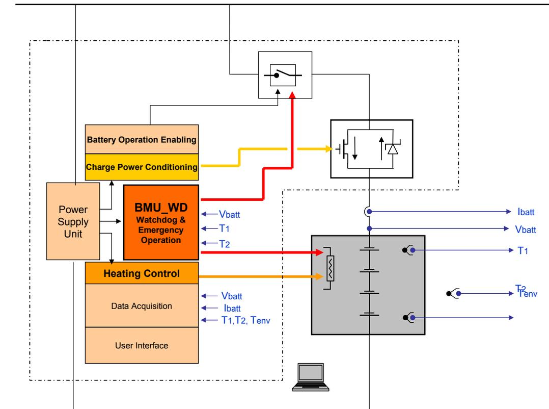
**Fig. 4 - Block Diagram of the SMS for SMC battery.**
