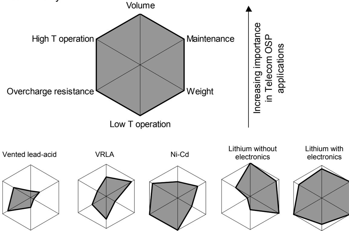
Figure 2 – Relative merits of various technologies for telecom OSP applications
