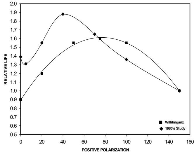
**Figure 1 – Relative life of vented lead-acid batteries as a function of positive plate polarization**
