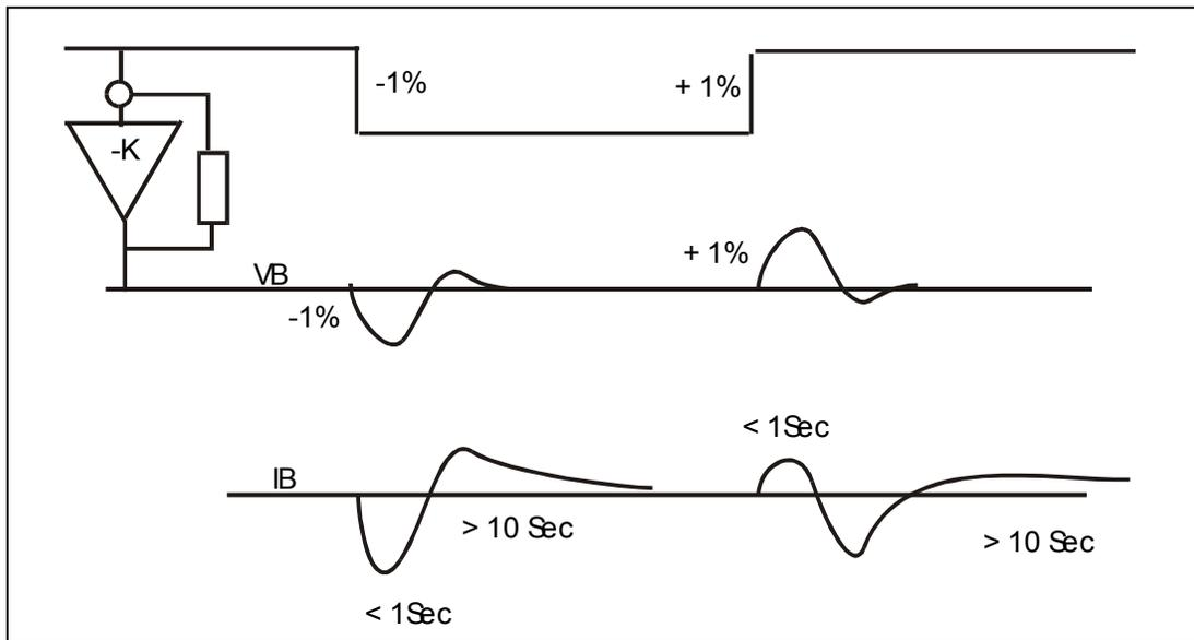
Fig. 6 Response of the high stability charger to the input voltage variation and resulting battery current
