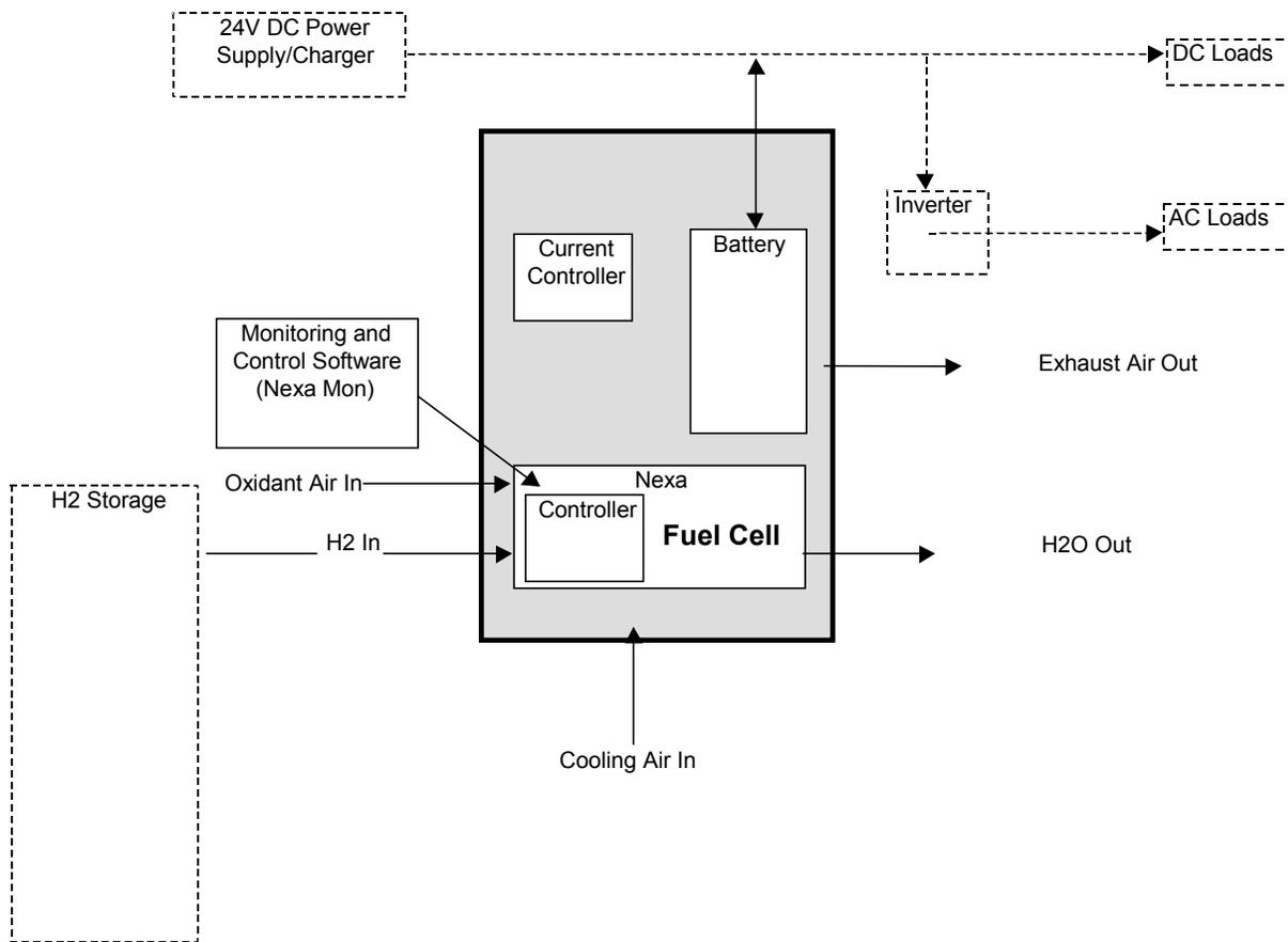
**Figure 2. Block Diagram of Battery and Hydrogen Fuel Cell System**
