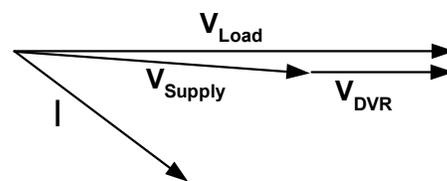
**Voltage Restoration<sup>3</sup>: Figure 8a. With Reactive Power Only**
