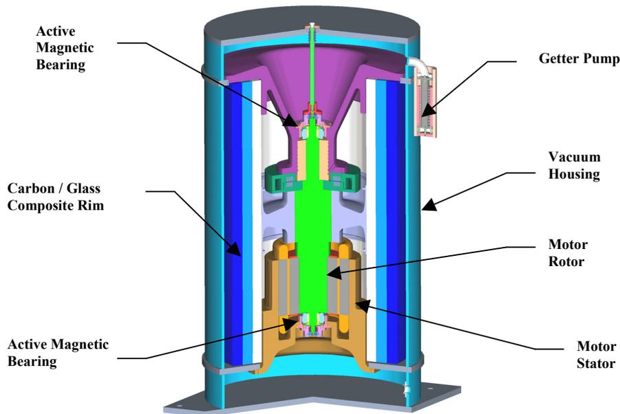
**Figure 3. High-Energy, High-Speed Flywheel Assembly**
