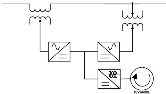
**Figure 13. Unified Power Flow Controller (UPFC)**
