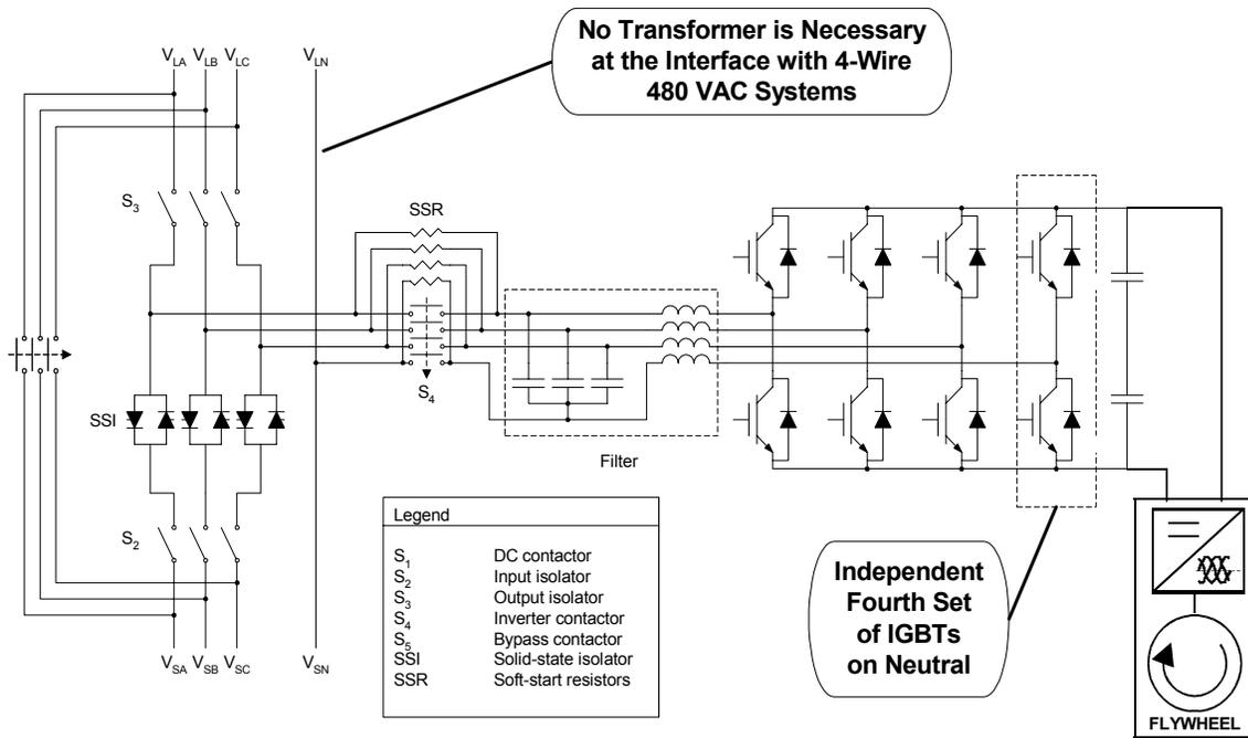
**Figure 12. Flywheel Supported Power Quality Compensator at 480 Volts**
