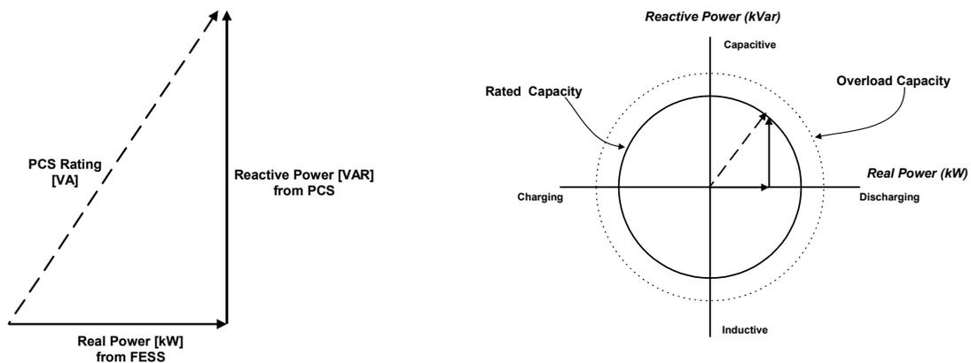
**Figure 7. Real/Reactive Power Vectors and Vector Space<sup>2</sup>**
