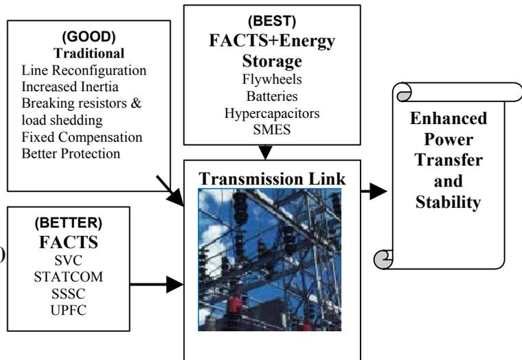
**Figure 14. The Ultimate Solution: FACTS+ESS<sup>4</sup>**
