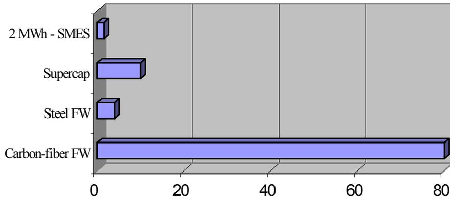
Figure 1. Stored Energy Density [Wh/kg] for Various Technologies<sup>1</sup>
