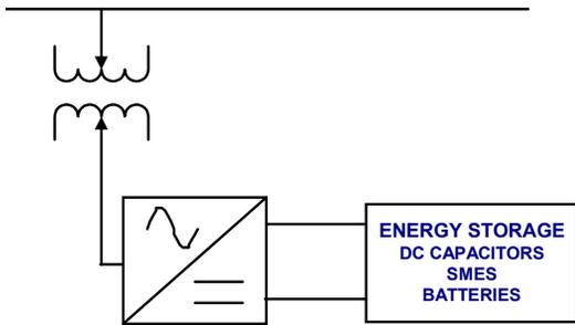
DSTATCOM Supported by: Figure 10a. Conventional Storage
