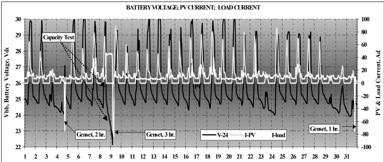
Figure 8. Battery Voltage, PV Current, and Load Current
