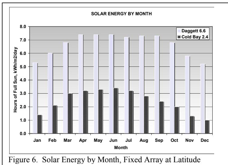
Figure 6. Solar Energy by Month, Fixed Array at Latitude
