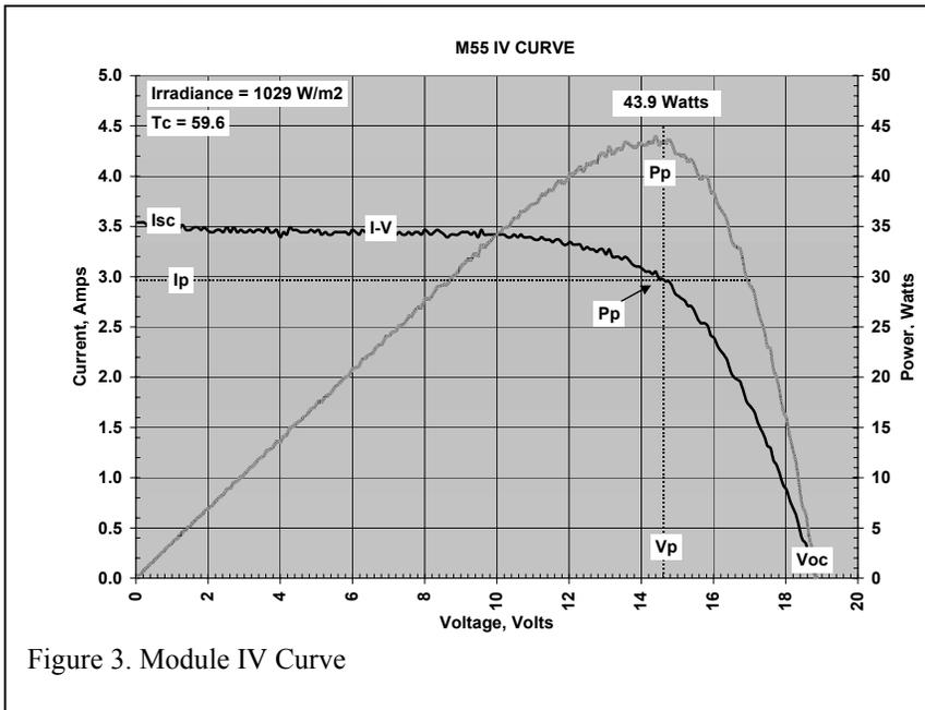
Figure 3. Module IV Curve
