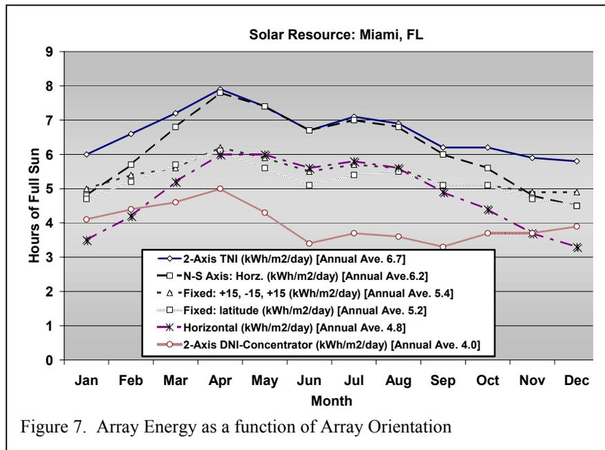
Figure 7. Array Energy as a function of Array Orientation
