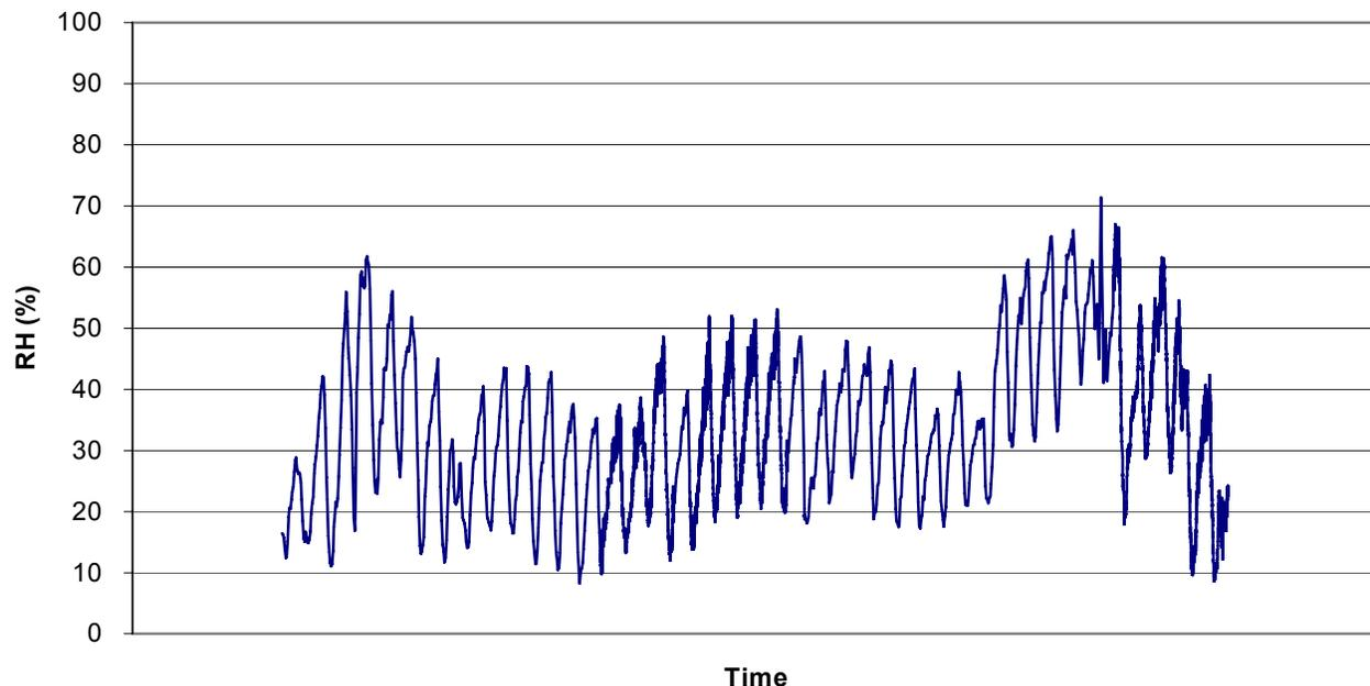
**FIGURE E.** The measured RH inside the battery compartment at site P. For this 3 month period, the average RH was 33%.
