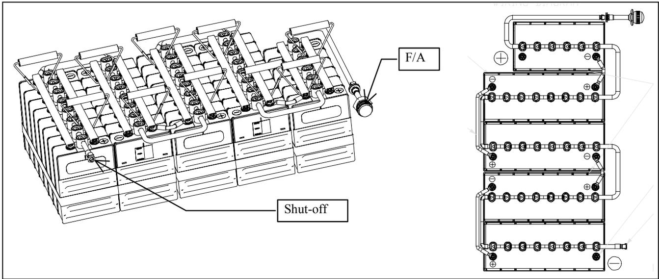
**FIGURE A. An example NCX battery string. Comprised of electrically and hydraulically interconnected blocks or modules, the 38 cell string operates on a typical 48V telecom buss. A single flame arrestor (F/A) is installed on the (+) side of the string for single point gas exhaustion and explosion protection.**
