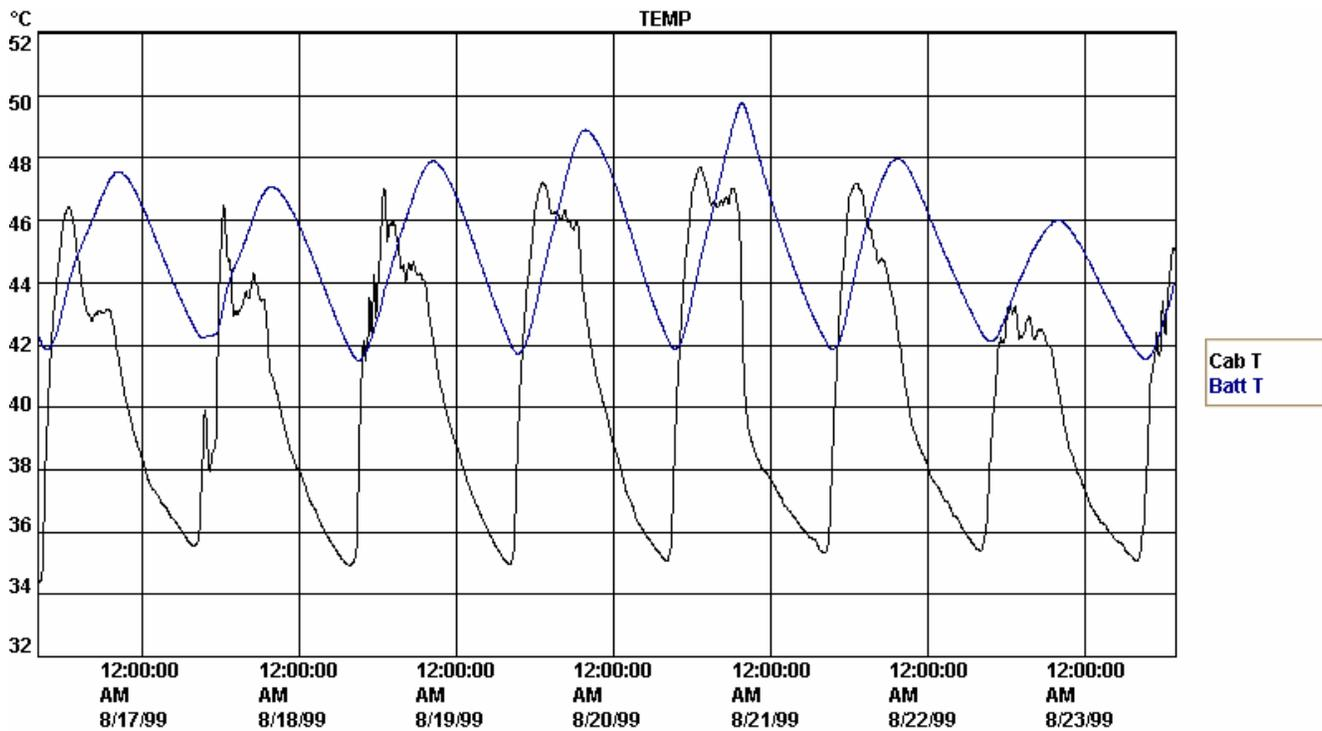
**FIGURE D. The measured battery string and cabinet temperature at site H. This one week period illustrates the operating temperature during the hottest time of the year. The average battery temperature is higher since it is installed in the highest or the hottest part of the cabinet and the cabinet temperature is measured in the lowest.**
