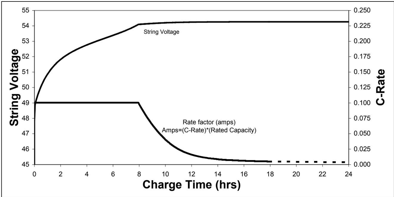
FIGURE B. The typical re-charge characteristics of an NCX type telecom battery string. At time zero the battery string is completely discharged. The max. voltage setting = 54.35 VDC, max. available current = 0.1C (12.5 Amps for NCX125 where C=125) and the temperature was ambient room. After 24 hrs, the string is ‘fully’ charged and ‘float charging’. Water is only consumed during this period of over-charging.
