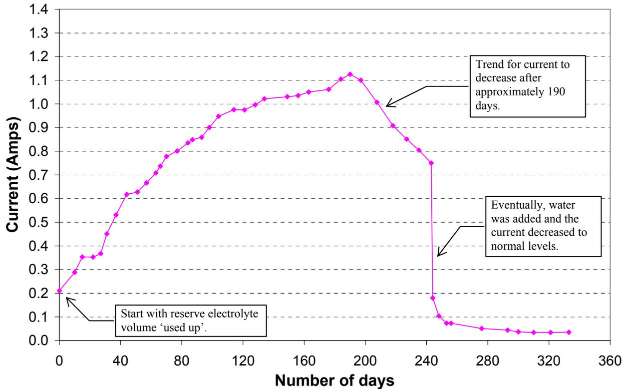
**FIGURE F. The current evolution of a Ni-Cd while under ‘starved’ electrolyte conditions. The test was conducted at 50°C (122°F) and with a fixed voltage of 1.43 V/cell (54.4 V for a 38 cell string typically used for a 48V telecom application).**
