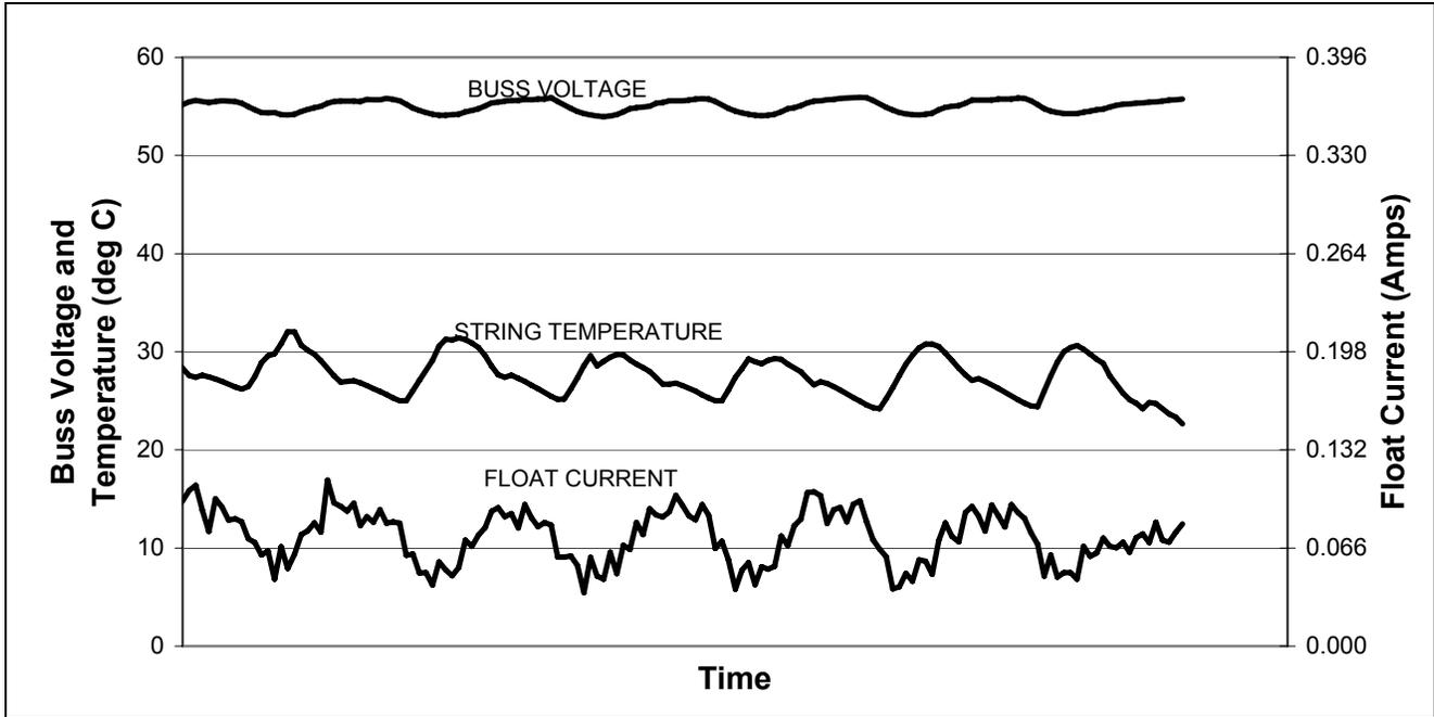
FIGURE C. The measured float charge characteristics of an Ni-Cd battery string installed in trial site #P (see Table A). Float current variations are a result of the temperature and buss voltage fluctuations.
