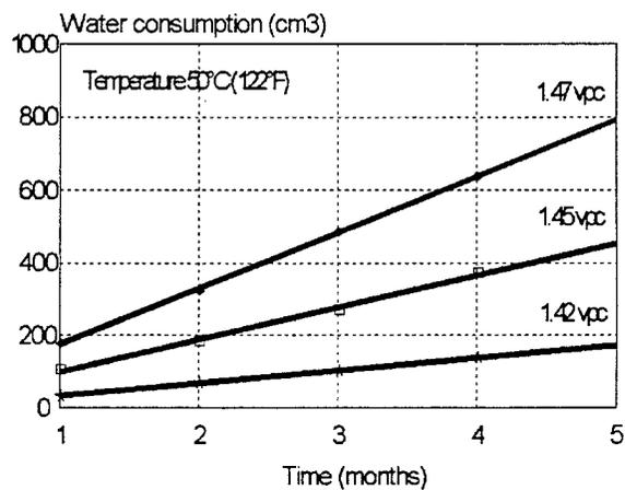
Figure 2 : Water consumption at 50°C (122°F)
