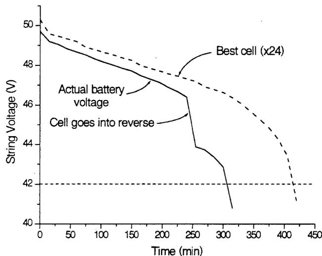
Figure 3 - Battery test results
