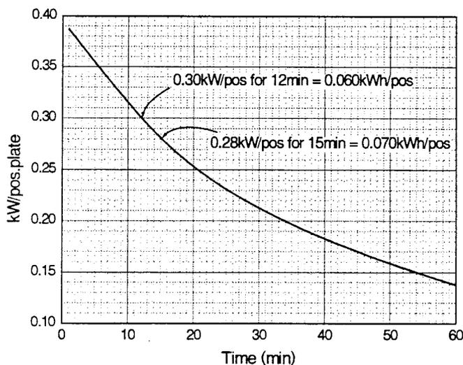
Figure 2 - Performance of Typical UPS Battery, kW/Positive Plate to 1.67V/cell
