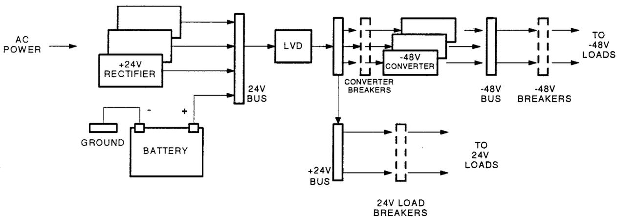
Figure 2 – Low Voltage Disconnect in Series with the Load
