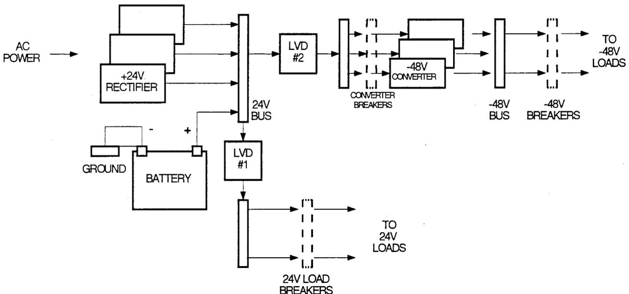
Figure 3 – Low Voltage Disconnect in a Load-Shed Configuration
