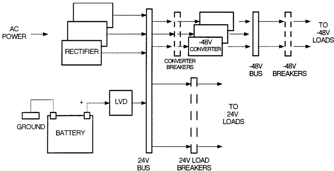
Figure 1 – Low Voltage Disconnect in Series with the Battery
