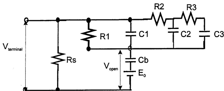
Figure 2. Battery Equivalent Circuitry
