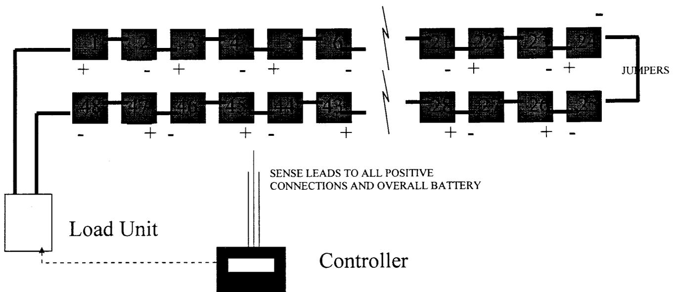
Battery strings with the same type cells but different voltages may be mixed as long as the combined string voltage is within the limits of the load units.
